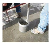
**Vibrating Concrete in Measure**
