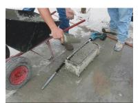
Making Beams Internal Vibration
