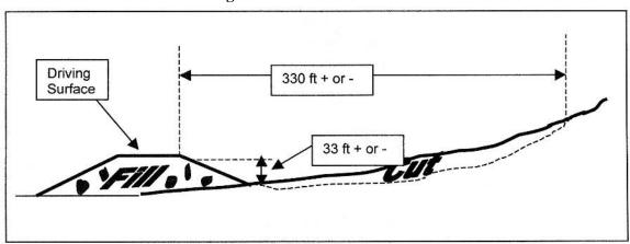
**Figure 8: Elevated Fill Section**
