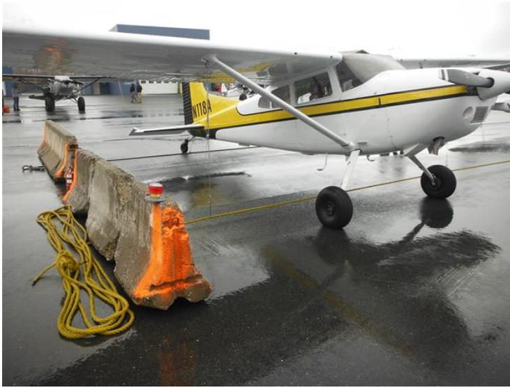
An alternative tie down system that allows cables to be anchored to an embedded engineered system would be beneficial. This alternative would remove the Jersey Barrier hazard to taxiing aircraft.
