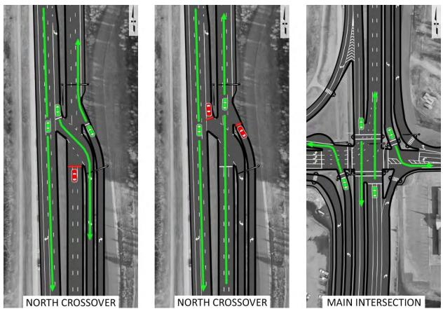
Figure 36: Alternative D – Vehicular Movements
