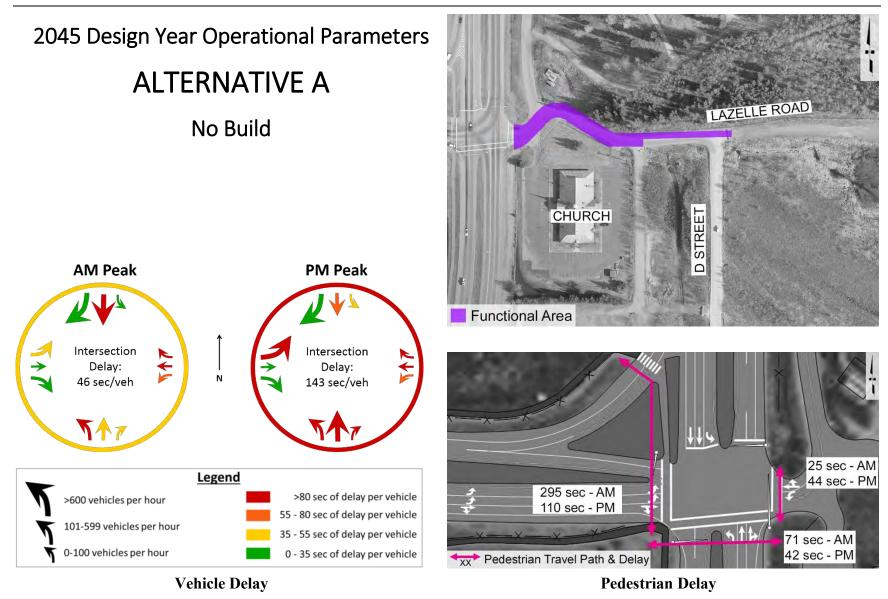
Figure 18: Operational Parameters for Alternative A, No Build
