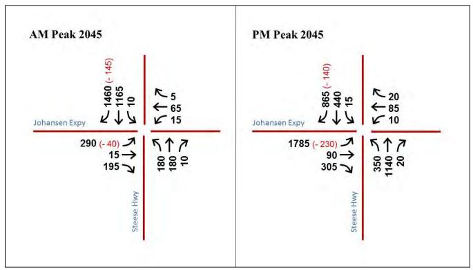
Figure 44: Design Turning Movement Volumes for Alternative E under Normal Growth
