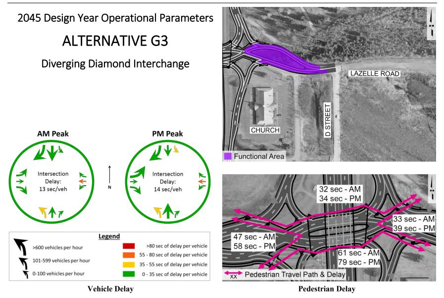
Figure 74: Operational Parameters for Alternative G3, Diverging Diamond Interchange
