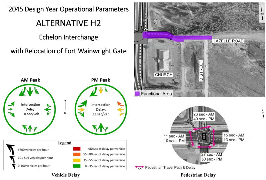
Figure 88: Operational Parameters for Alternative H2, Partial Echelon Interchange with Relocation of Fort Wainwright Gate
