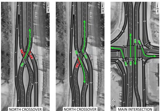
Figure 29: Alternative C – Vehicular Movements
