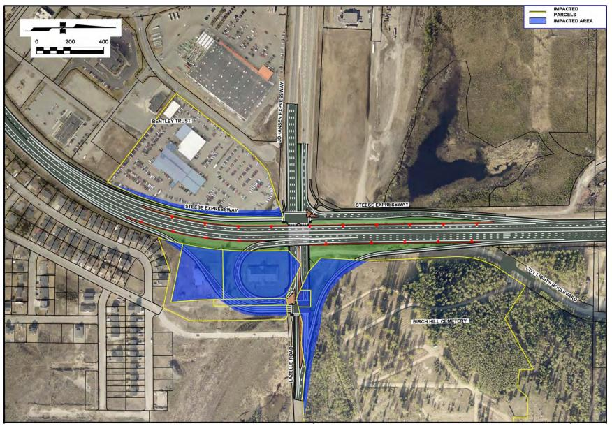
Figure 71: ROW Impacts for Alternative G2, Diamond Interchange with Cloverleaf Ramp
