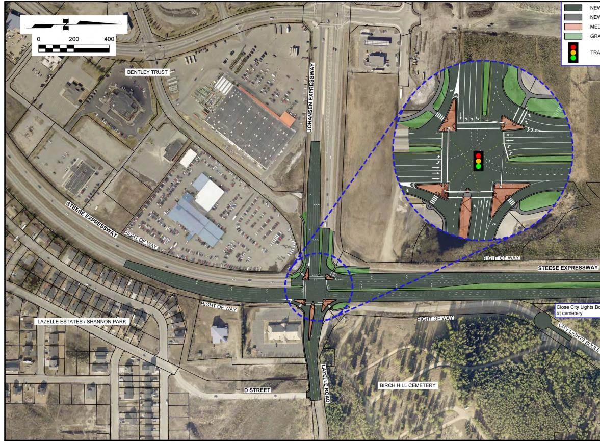
Figure 21: Alternative B – Conventional Intersection with Relocation of Fort Wainwright Gate
