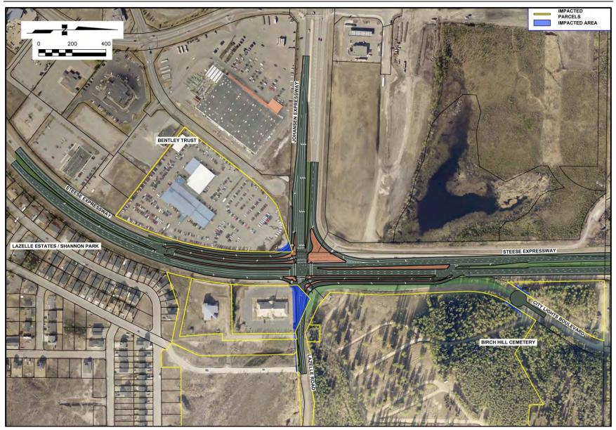
Figure 41: ROW Impacts for Alternative D, Partial Displaced Left Turn Intersection
