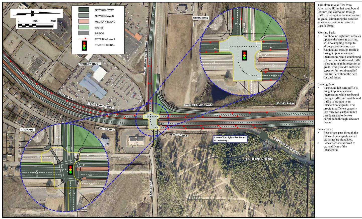
Figure 85: Alternative H2 – Partial Echelon Interchange
