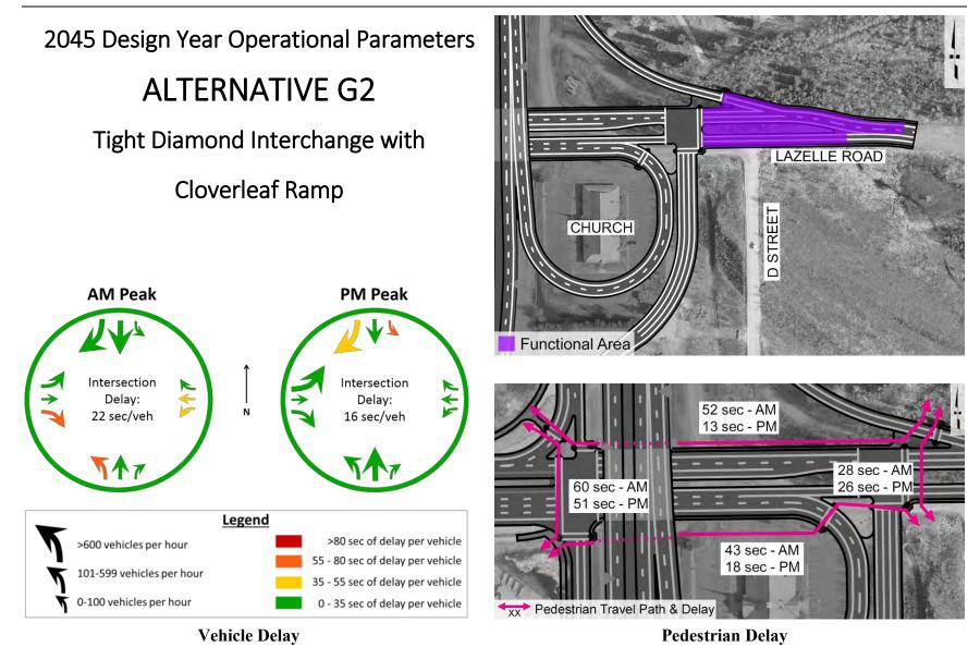
Figure 67: Operational Parameters for Alternative G2, Tight Diamond Interchange with Cloverleaf Ramp
