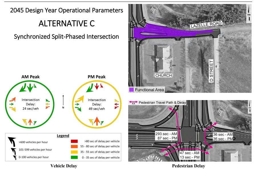
Figure 30: Operational Parameters for Alternative C, Synchronized Split-Phased Intersection
