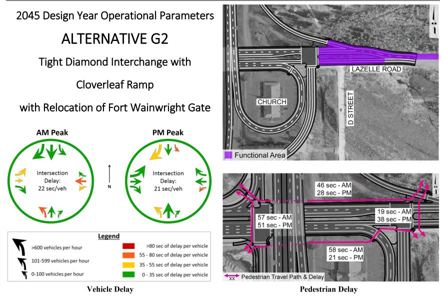
Figure 69: Operational Parameters for Alternative G2, Tight Diamond Interchange with Cloverleaf Ramp with Relocation of Fort Wainwright Gate
