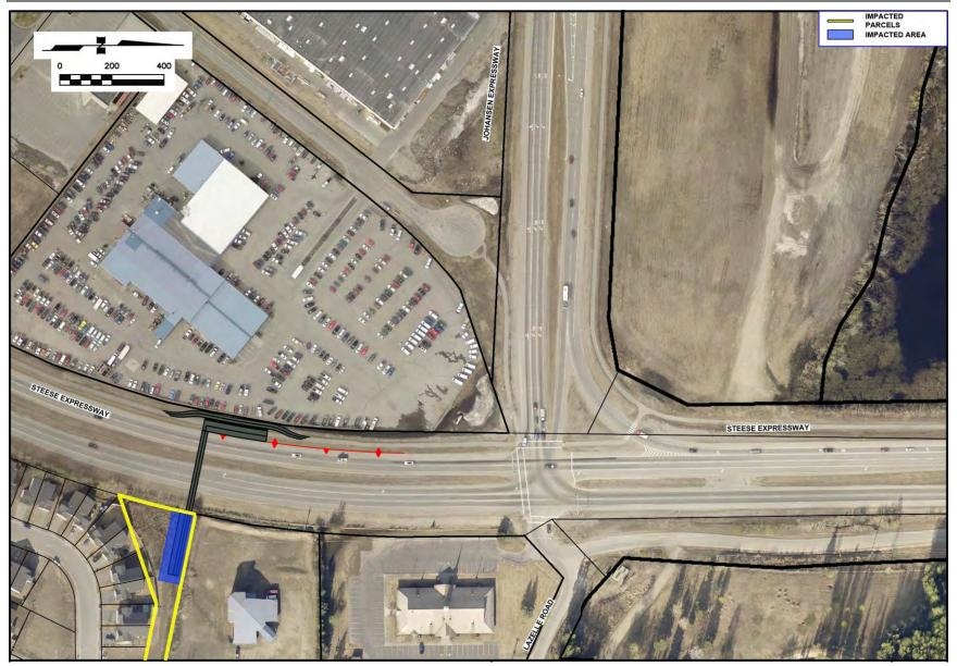
Figure 92: ROW Impacts for Alternative I, Pedestrian Overpass
