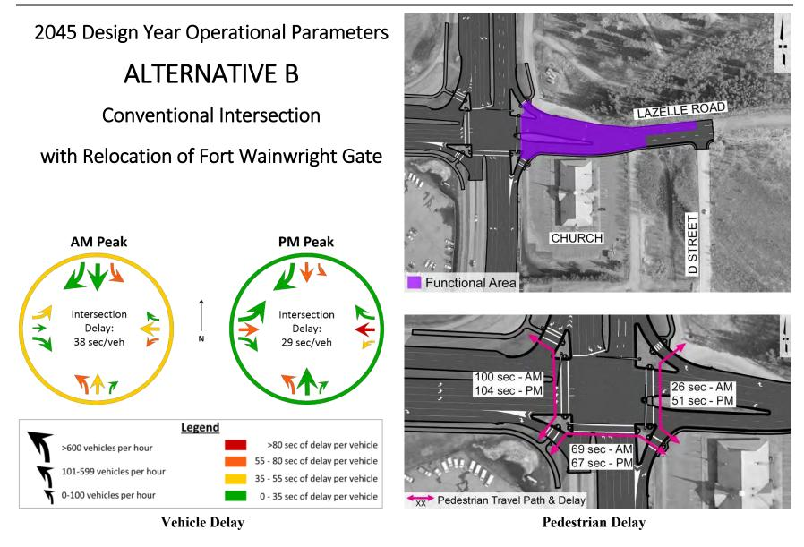
Figure 24: Operational Parameters for Alternative B, Conventional Intersection with Relocation of Fort Wainwright Gate
