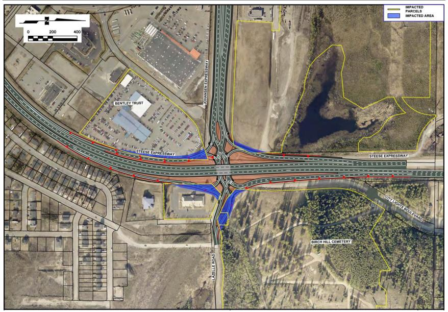
Figure 78: ROW Impacts for Alternative G3, Diverging Diamond Interchange
