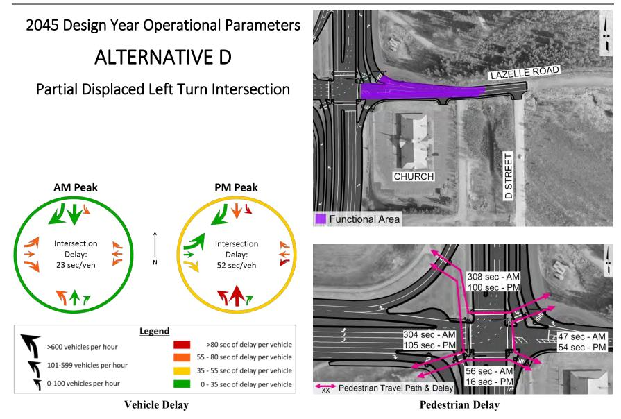
Figure 37: Operational Parameters for Alternative D, Partial Displaced Left Turn Intersection
