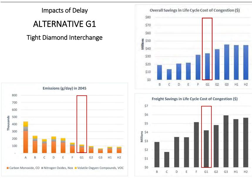
Figure 62: Impacts of Delay for Alternative G1, Tight Diamond Interchange
