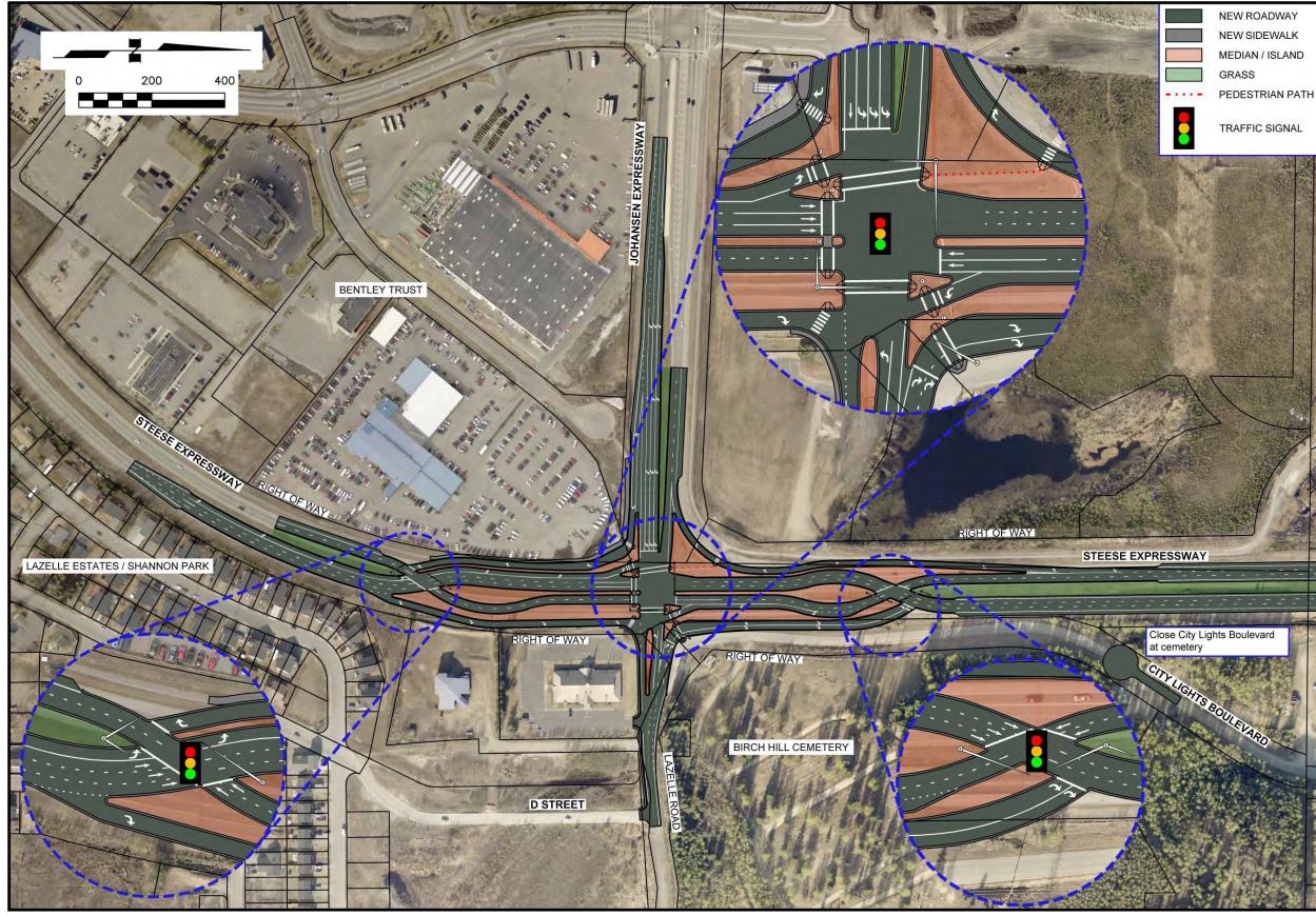
Figure 28: Alternative C – Synchronized Split-Phased Intersection
