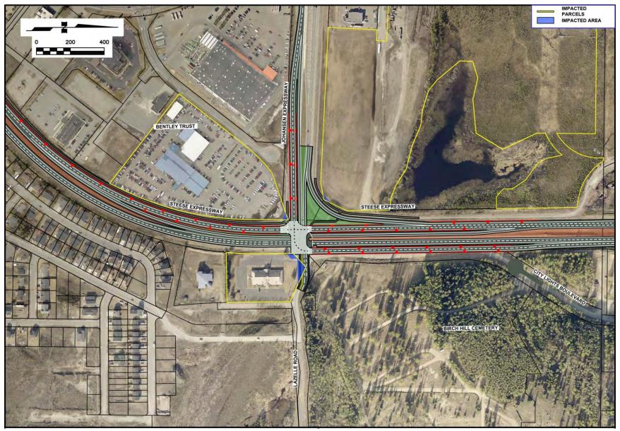
Figure 90: ROW Impacts for Alternative H2, Partial Echelon Interchange
