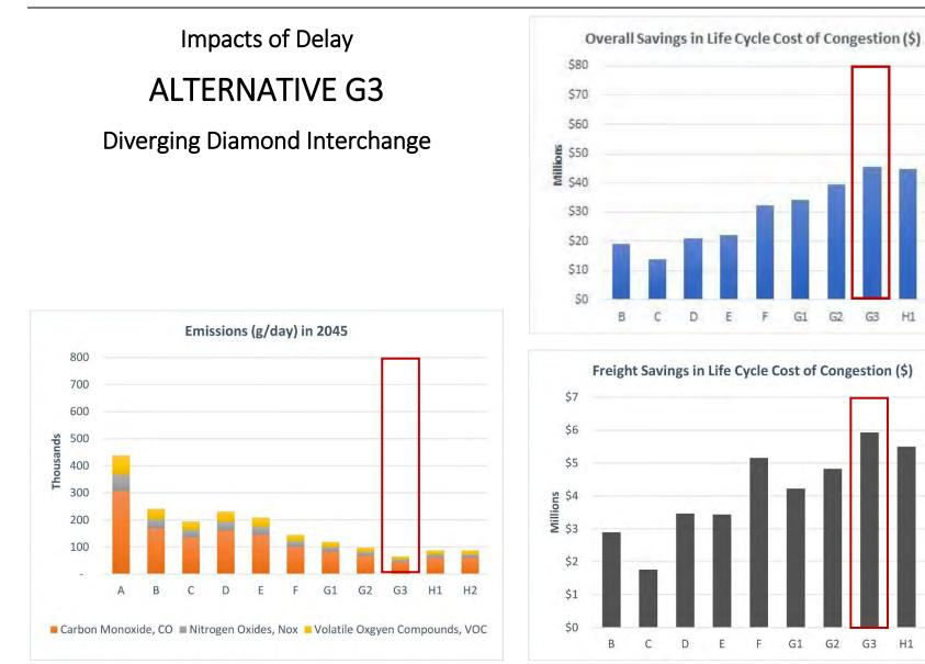
Figure 75: Impacts of Delay for Alternative G3, Diverging Diamond Interchange
