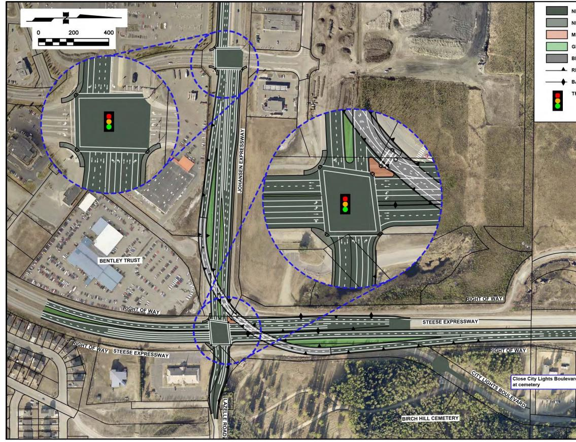
Figure 53: Alternative F – Eastbound Left Turn Flyover with Relocation of Fort Wainwright Gate
