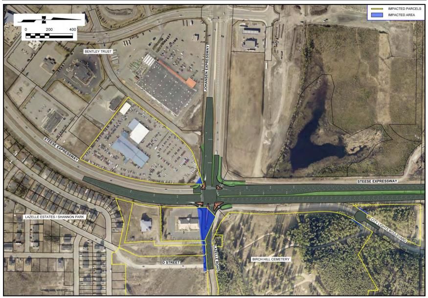
Figure 27: ROW Impacts for Alternative B, Conventional Intersection with Relocation of Fort Wainwright Gate
