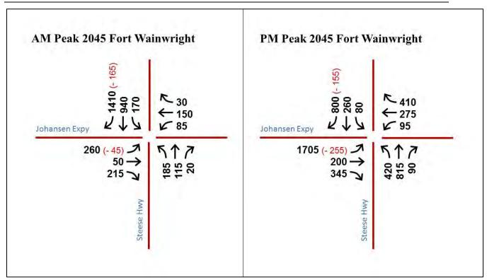
Figure 45: Design Turning Movement Volumes for Alternative E with Relocation of Fort Wainwright Connection
