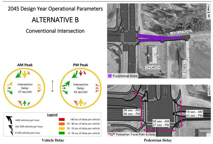
Figure 22: Operational Parameters for Alternative B, Conventional Intersection
