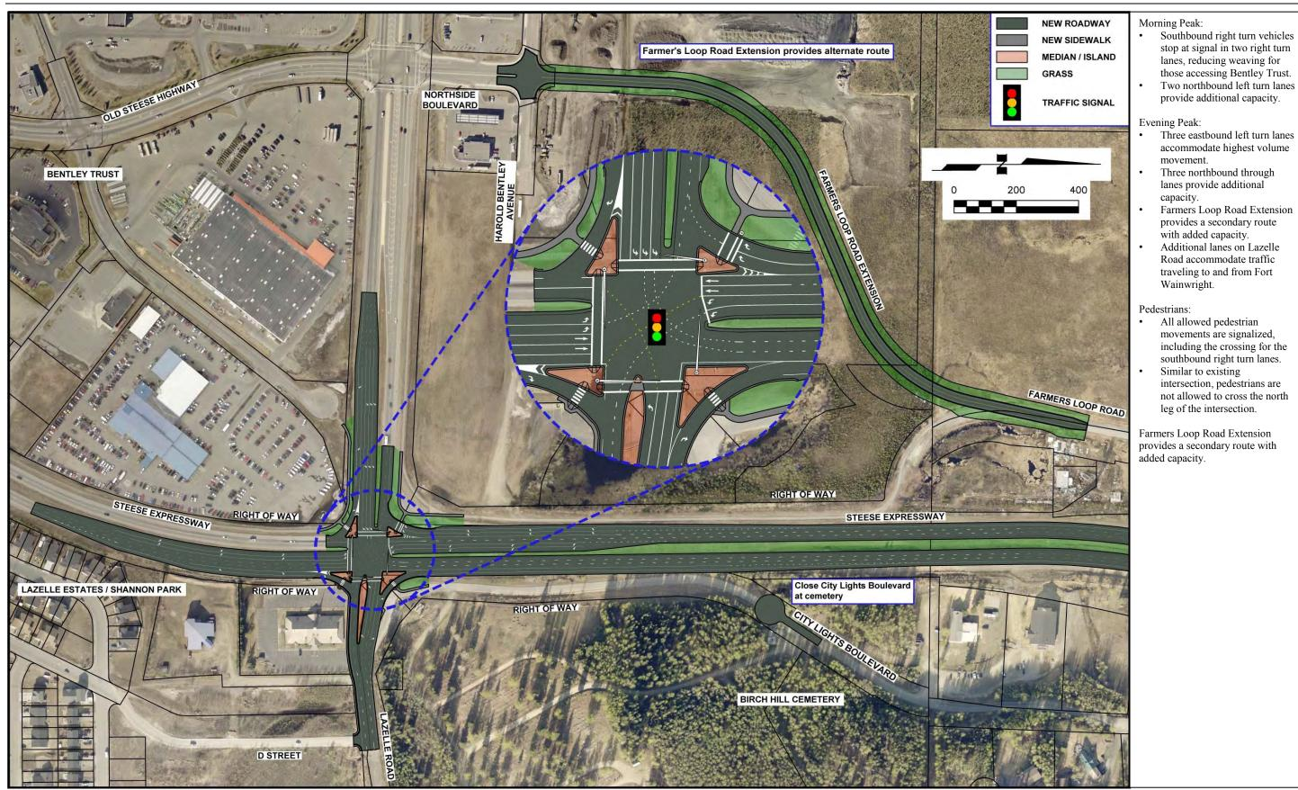
Figure 43: Alternative E – Old Steese to Farmers Loop Connection with Relocation of Fort Wainwright Gate
