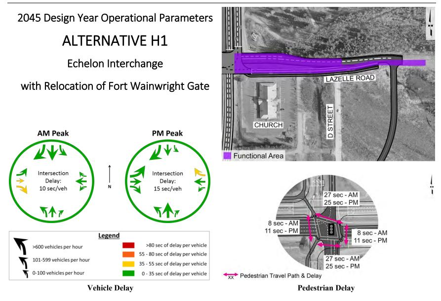
Figure 82: Operational Parameters for Alternative H1, Echelon Interchange with Relocation of Fort Wainwright Gate
