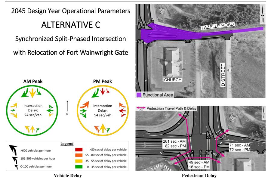
Figure 32: Operational Parameters for Alternative C, Synchronized Split-Phased Intersection with Relocation of Fort Wainwright Gate
