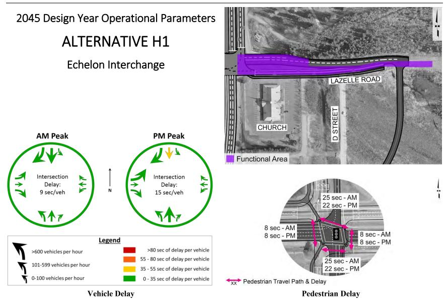
Figure 80: Operational Parameters for Alternative H1, Echelon Interchange
