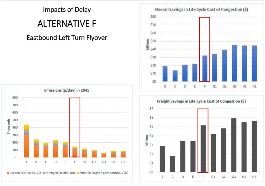
Figure 55: Impacts of Delay for Alternative F, Eastbound Left Turn Flyover
