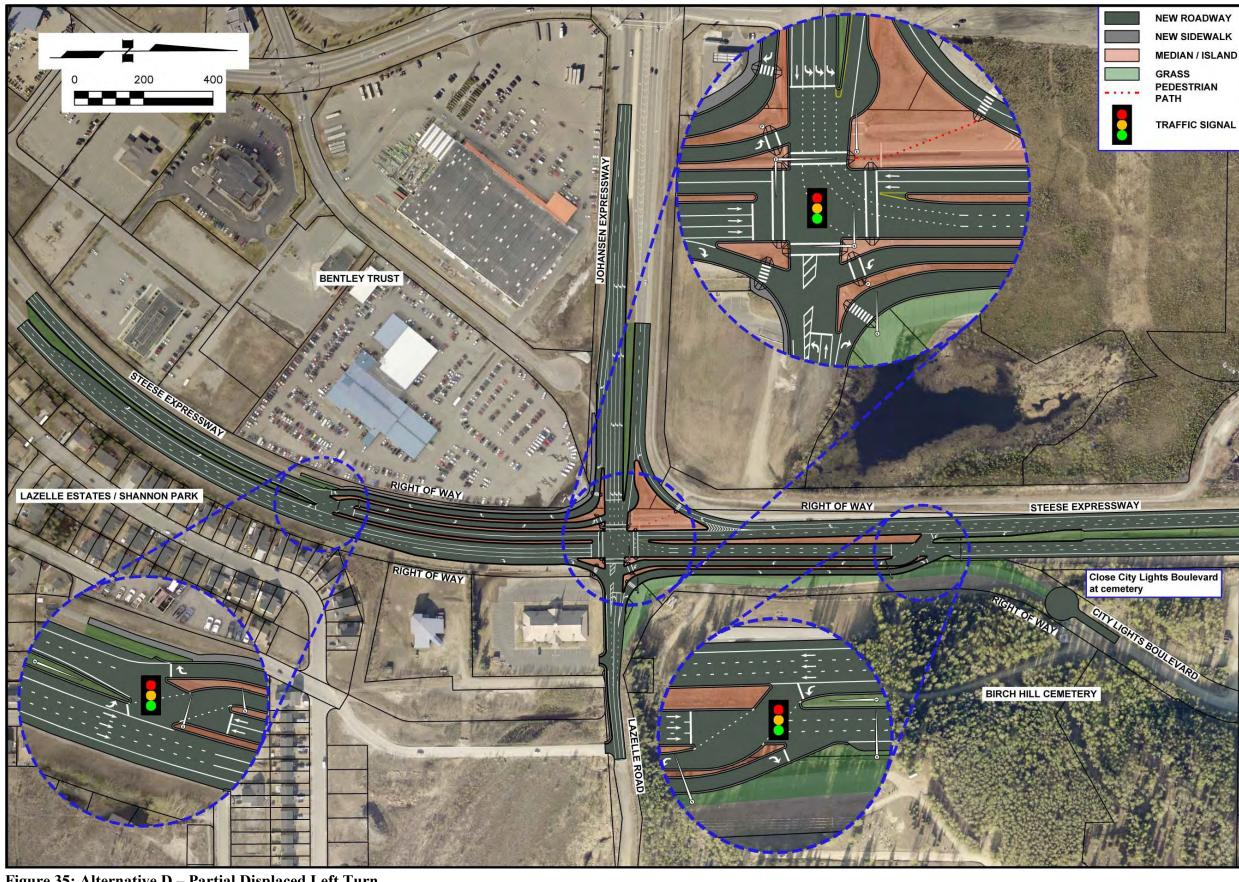
Figure 35: Alternative D – Partial Displaced Left Turn
