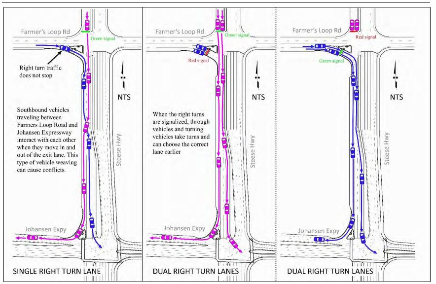
Figure 13: Farmers Loop Conversion of Free Right Turn Lane to Signalized Dual Lanes
