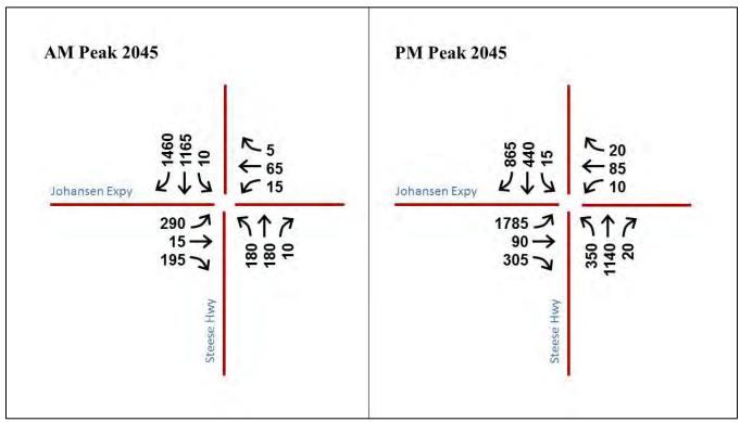
Figure 16: Design Turning Movement Volumes under Normal Growth
