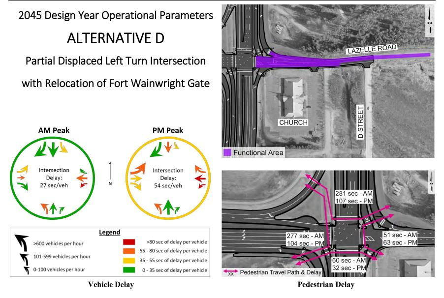
Figure 39: Operational Parameters for Alternative D, Partial Displaced Left Turn Intersection with Relocation of Fort Wainwright Gate
