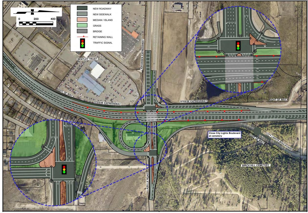
Figure 66: Alternative G2 – Tight Diamond Interchange with Cloverleaf Ramp
