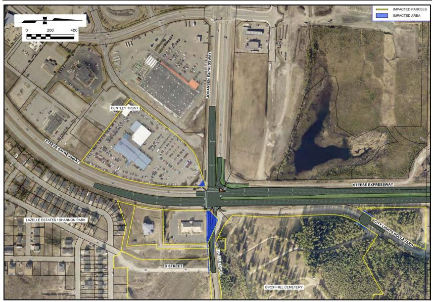
Figure 26: ROW Impacts for Alternative B, Conventional Intersection
