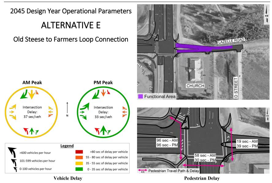
Figure 46: Operational Parameters for Alternative E, Old Steese to Farmers Loop Connection
