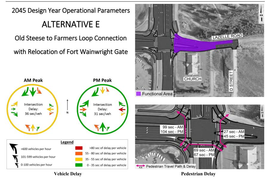
Figure 48: Operational Parameters for Alternative E, Old Steese to Farmers Loop Connection with Relocation of Fort Wainwright Gate
