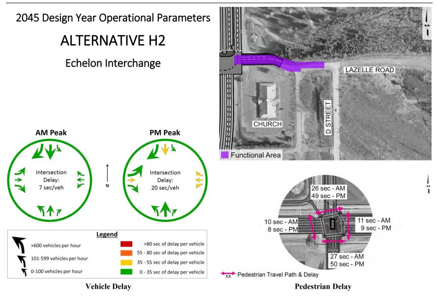
Figure 86: Operational Parameters for Alternative H2, Partial Echelon Interchange
