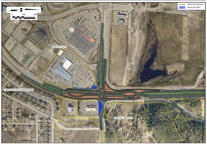
Figure 34: ROW Impacts for Alternative C, Synchronized Split-Phased Intersection
