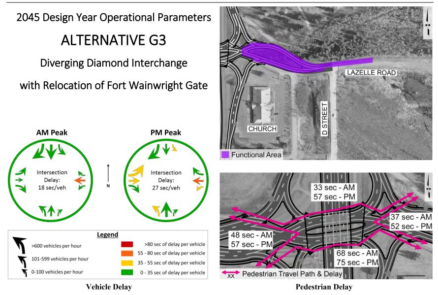
Figure 76: Operational Parameters for Alternative G3, Diverging Diamond Interchange with Relocation of Fort Wainwright Gate
