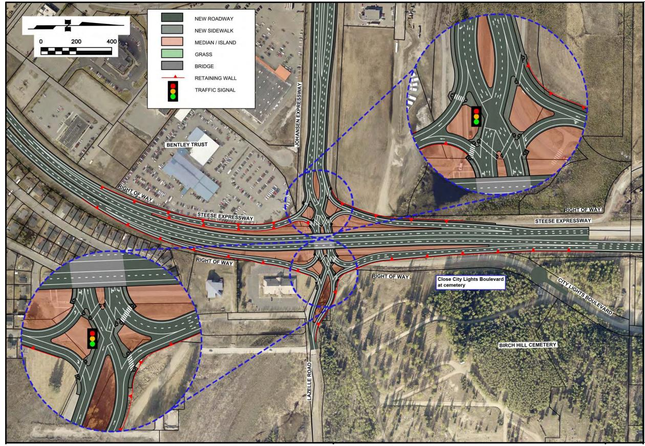
Figure 72: Alternative G3 – Diverging Diamond Interchange
