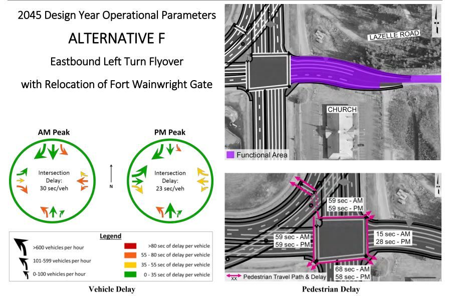
Figure 56: Operational Parameters for Alternative F, Eastbound Left Turn Flyover with Relocation of Fort Wainwright Gate
