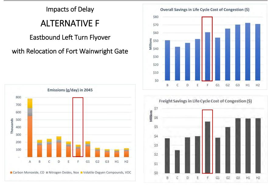
Figure 57: Impacts of Delay for Alternative F, Eastbound Left Turn Flyover with Relocation of Fort Wainwright Gate
