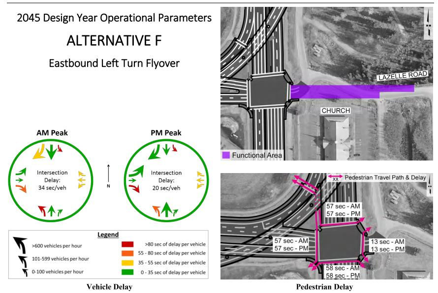
Figure 54: Operational Parameters for Alternative F, Eastbound Left Turn Flyover
