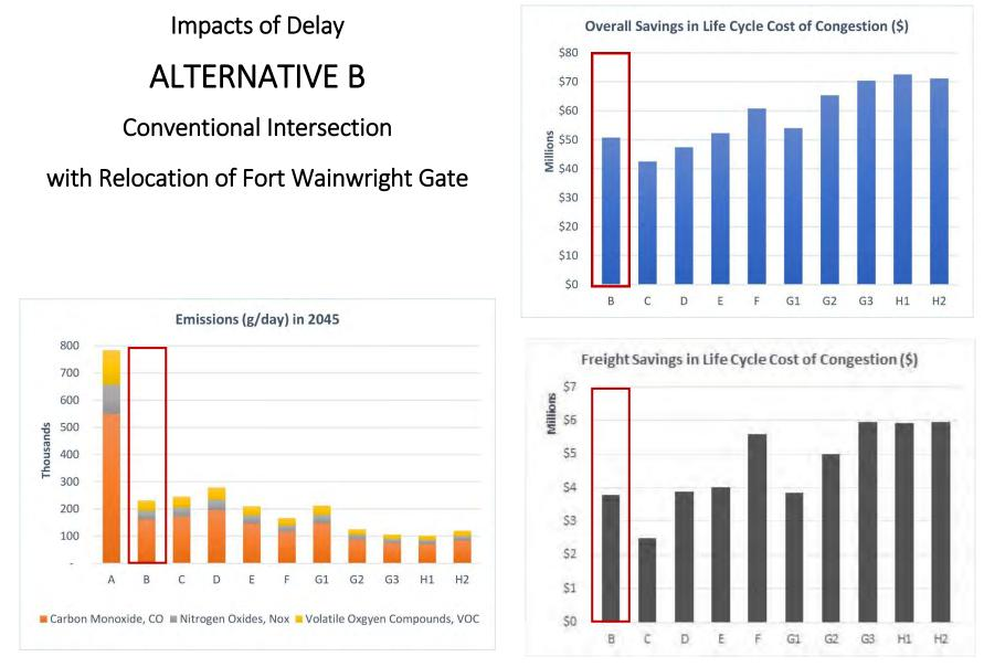
Figure 25: Impacts of Delay for Alternative B, Conventional Intersection with Relocation of Fort Wainwright Gate
