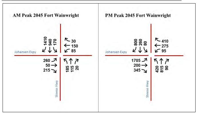
Figure 17: Design Turning Movement Volumes with Relocation of Fort Wainwright Main Gate
