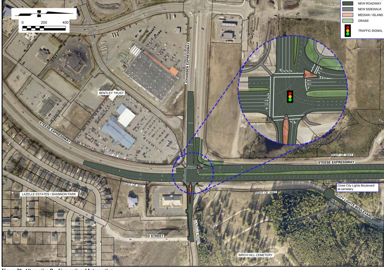
Figure 20: Alternative B – Conventional Intersection
