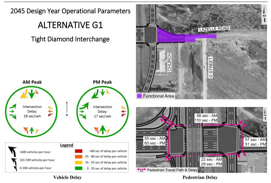
Figure 61: Operational Parameters for Alternative G1, Tight Diamond Interchange
