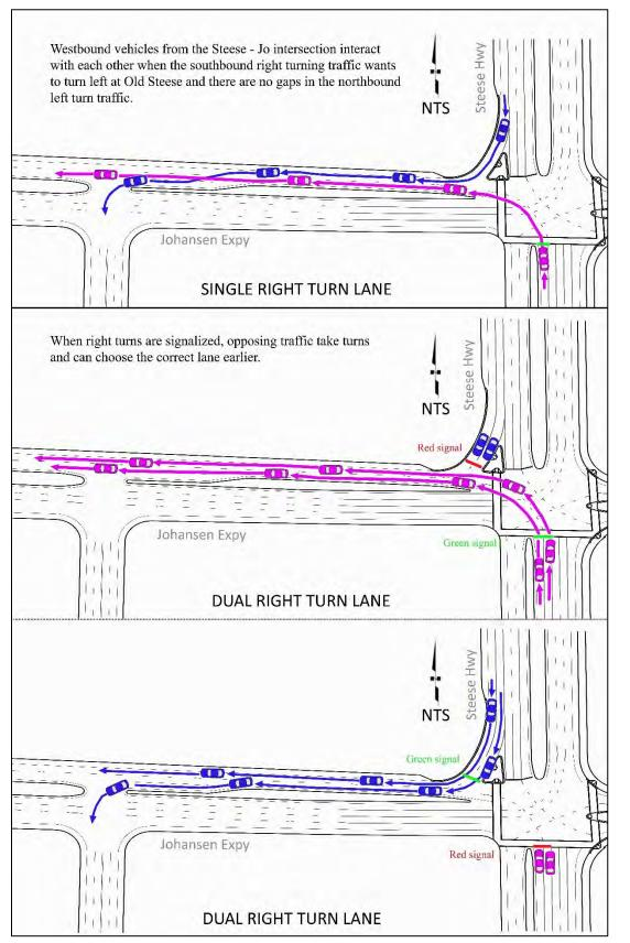
Figure 14: Steese-Jo Conversion of Free Right Turn Lane to Signalized Dual Lanes
