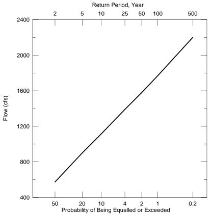
Figure 2. Estimated discharge and exceedance probability for new bridge at Kuchoruk Creek near Noatak, Alaska.
