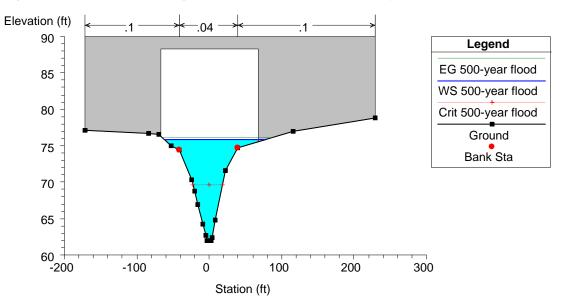
Figure 3. Kuchoruk Creek Bridge Cross Section Model Output, 500-year Flood, Alternative 1.
