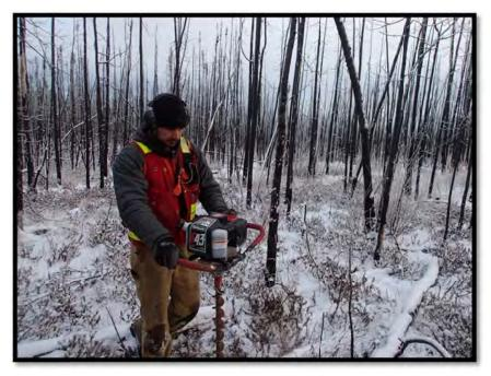
*Photo* 0097 – gas-powered auger used for geotechnical sampling
