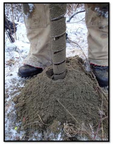
*Photo* 0058 – *Typical clean sand found underlying the silt layer.*
