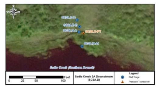
FIGURE 2.7: HYDROLOGIC STAFF GAGES INSTALLED AT SC2A.D
