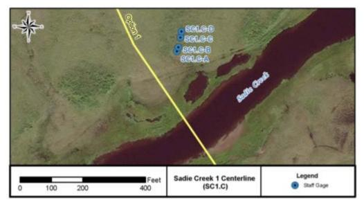
FIGURE 2.3: HYDROLOGIC STAFF GAGES INSTALLED AT SC1.C
