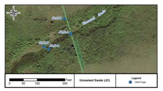
FIGURE 2.9: HYDROLOGIC STAFF GAGES INSTALLED AT JC
