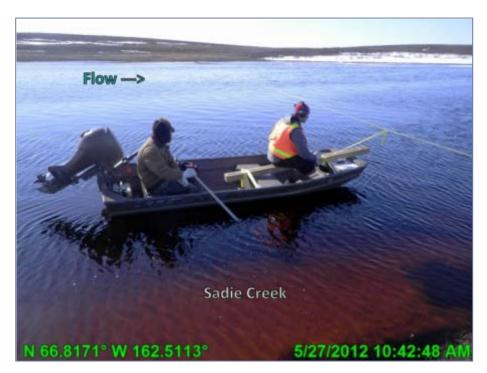
PHOTO 3.3: DIRECT-DISCHARGE MEASUREMENT AT SC1, LOOKING SOUTHEAST; MAY 27, 2012
