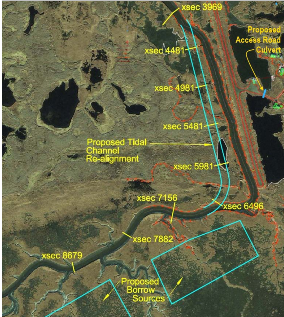
Figure 4. Proposed tidal channel realignment and HEC-RAS cross-sections.
