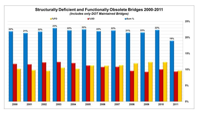
Figure 2. Structurally Deficient and Functionally Obsolete Bridges DOT-Owned Only
